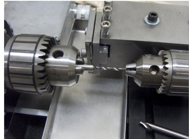
Drilling of inner Pt capsule in preparation for acid leaching
