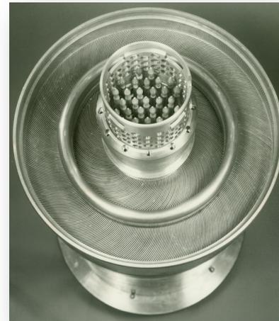
Target positions shown occupied in this HFIR reactor core mock-up
