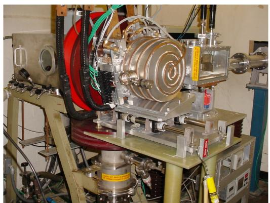
Internal vacuum system is radiologically contaminated from years of testing targets and ion sources for RIB production (some areas of the target room are off-limits) There are electrical hazards (e.g. high current and high voltage) around the TIS enclosure platform.
