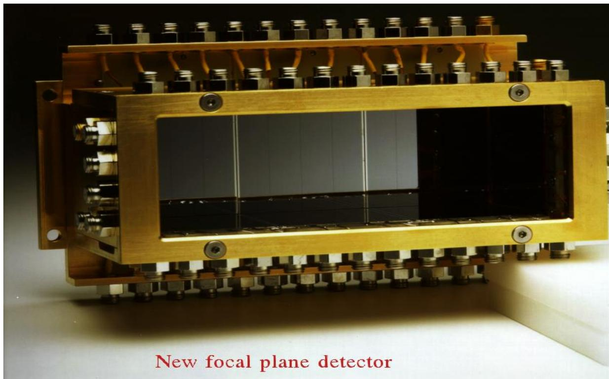
The addition of the top, bottom, and side detectors increased the geometry for counting  $\alpha$  particles from 50% to 87%. Veto detectors mounted behind the focal plane were used to identify and reject light charged particles passing through the separator.
