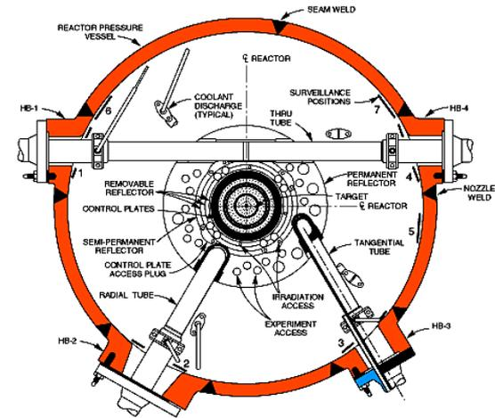
Sectional plan view of reactor core
