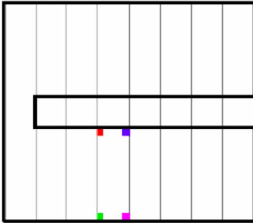
Principle: The movement of charge in a given segment induces a signal on the electrodes of neighbouring segments. The shape of this induced signal is sensitive to the spatial position of the  $\gamma$ -ray interaction point.
