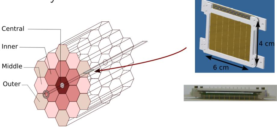
Auxiliary detectors include two 1 mm thick silicon strip detectors placed in the center of MTAS around the tape.
